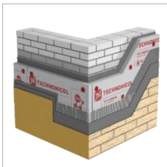
Fastening XPS on basement to decking
